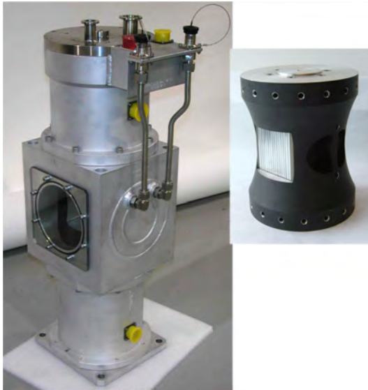
Figure 6.12: Left: photograph of ARCS Fermi chopper, showing housing, windows, and water cooling. Right: photograph of the slit package, with aluminum slits seen end-on.
