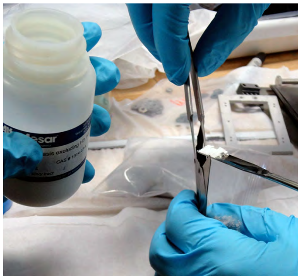
Figure 6.8: Loading powder into the sachet. For valuable powders it is appropriate to do the loading over clean aluminum foil so that any spilled powder can be recovered and reused.
