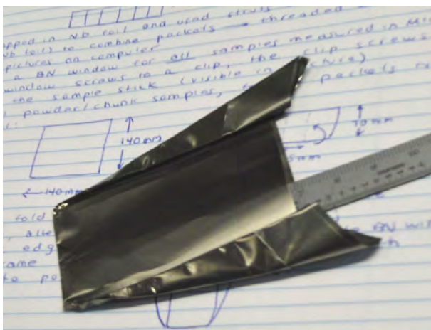
Figure 6.7: A partially-complete sachet. A sheet of thin niobium was folded in half, and the edges were folded multiple times in ever sharper triangle shapes. A pair of pliers will be used to crimp the edges.
