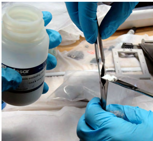
Figure 10.8: Loading powder into the sachet. For valuable powders it is appropriate to do the loading over clean aluminum foil so that any spilled powder can be recovered and reused.
