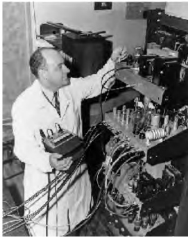
Figure 10.1: Enrico Fermi works with an electronic control for a neutron chopper during his Argonne days.
