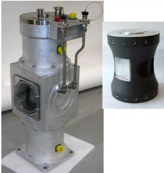
Figure 10.11: Left: photograph of ARCS Fermi chopper, showing housing, windows, and water cooling. Right: photograph of the slit package, with aluminum slits seen end-on.
