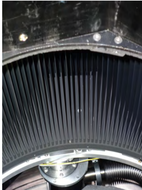
Figure 12.6: Photograph of the inner edge of collimator septa around the sample region of the ARCS spectrometer. The perspective of the photo is from a camera slightly above the position of the sample. The detector array lies approximately 2 m beyond the collimator towards the top of the photograph.
