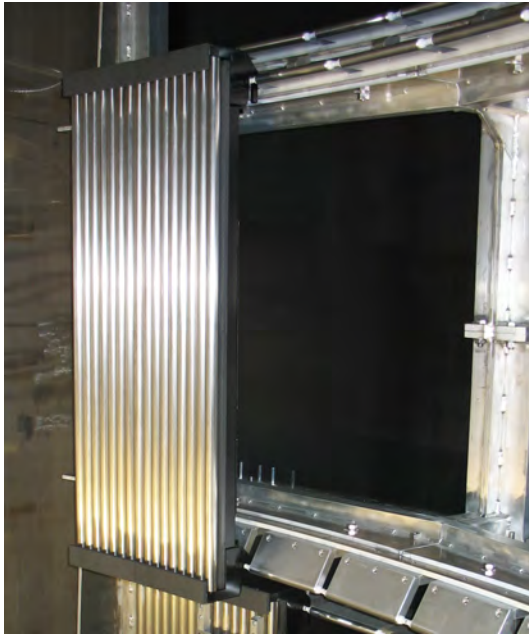
Figure 10.13: Installation of detector bank on the ARCS spectrometer, showing 16 tubes in the middle bank. Each tube is 1 m in height and approximately 2.5 cm in diameter.
