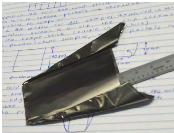
Figure 10.7: A partially-complete sachet. A sheet of thin niobium was folded in half, and the edges were folded multiple times in ever sharper triangle shapes. A pair of pliers will be used to crimp the edges.
